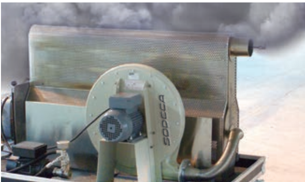
Smoke Machine for performing real smoke tests
